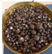
Figure 1: Appearance of pelletized synthetic aggregates after sintering.
