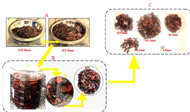
Figure 18: Durability test results of the aggregate according to DNIT 446/2024-ME.
